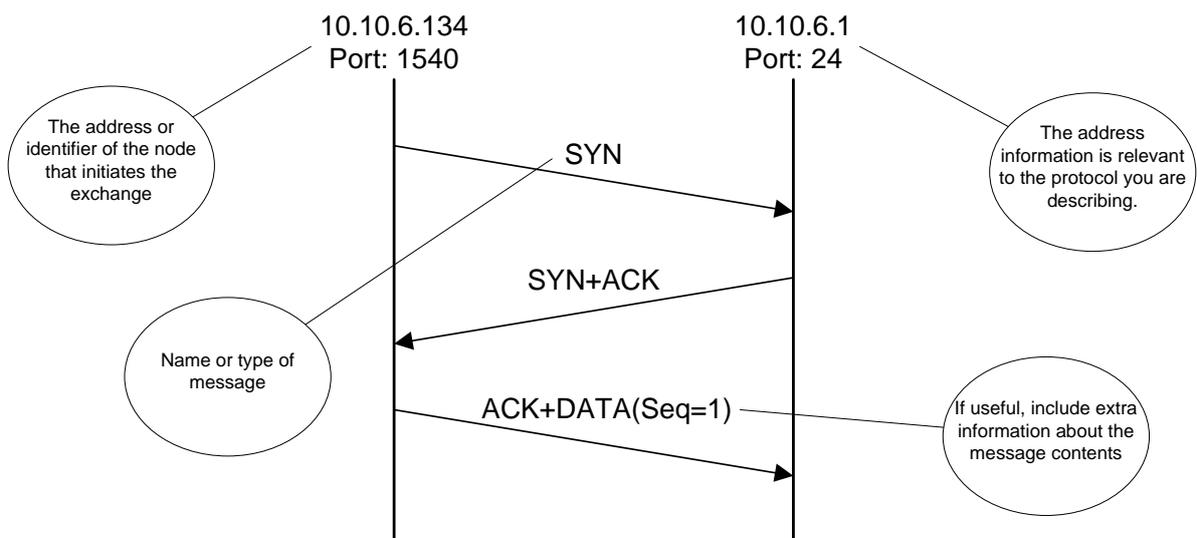
Figure 3: Example illustrating an exchange of packets
