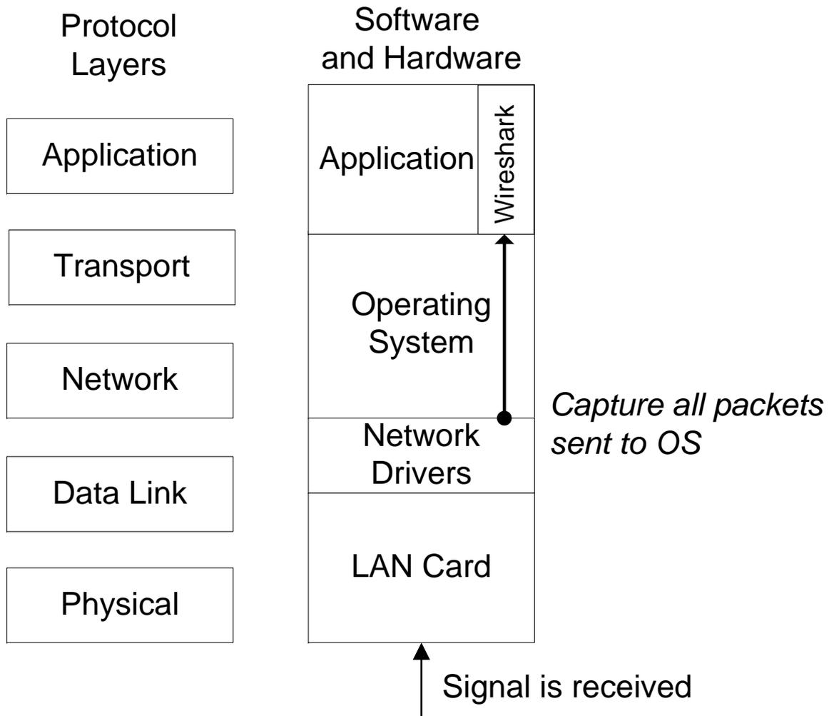
Figure 1: Capturing packets in the Operating System
