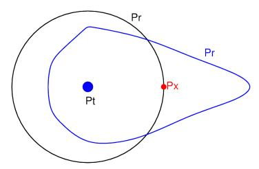
The gain of the blue directional antenna is the ratio between power received 1m away From directional antenna (Px) and power received 1m away from isotropic antenna (Pr)
