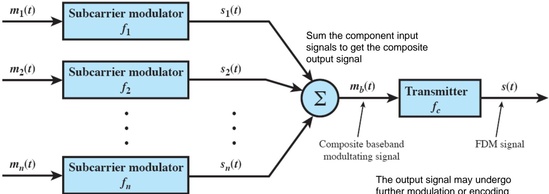
Modulate each signal onto a separate frequency (also remove components that are not necessary)
