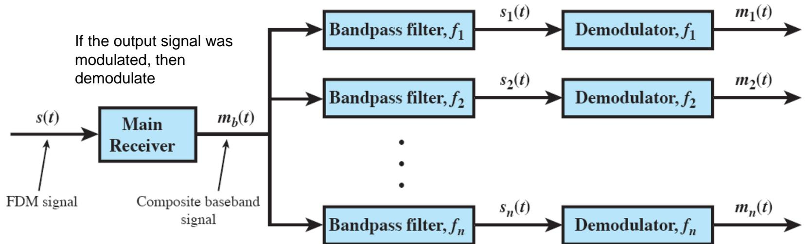
If the output signal was modulated, then demodulate
