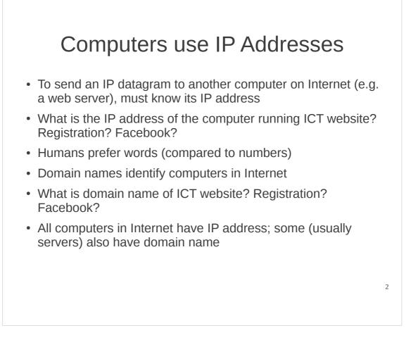
The core protocol for Internet communications is IP. To get data from one computer to another, IP is used. And importantly, the IP address of the destination computer is needed by the source (and intermediate routers) to correctly deliver the datagram. IP addresses identify computers (or more precisely, network interfaces on computers) in the Internet.
