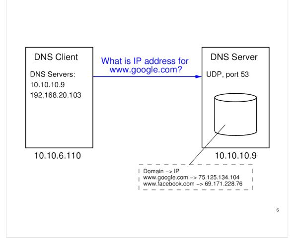
The DNS Resolver on 10.10.6.110 has the domain www.google.com. It wants to know the IP address of the computer that this domain identifies.
