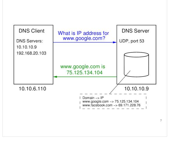
When the DNS server receives the query, it checks its database of mappings. In this example, the domain www.google.com is in the database. Therefore the DNS Server responds, indicating the IP address for the computer identified by the domain.
